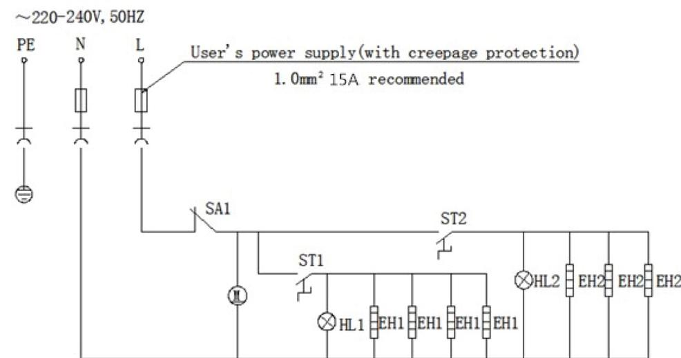
SA1: ON/OFF Switch      ST1/ ST 2: Thermostat      M:Motor
